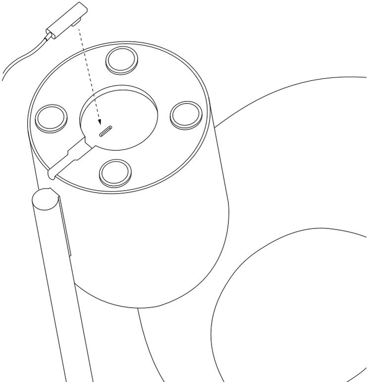
Insert cable in the bottom of the lamp to charge.
